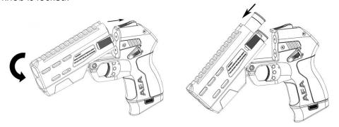
The safety device will not be able to pull the trigger at S. Move to F to launch.
